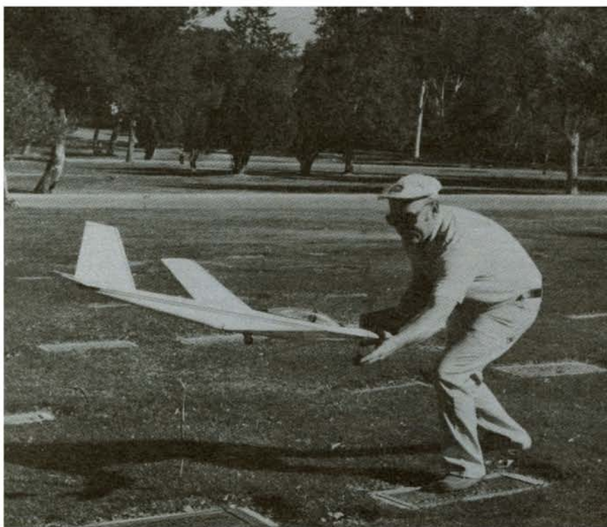
About to catch the Seville after a soaring flight is Bill Evans. Not only is this ship practical and simple, but it is enjoyably stable. The wing is foam cored, ply or balsa skin.
